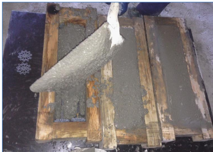
Moulds used to manufacture the laboratory sample
